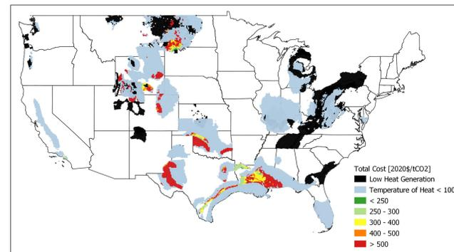
**Fig. 3: Geospatial Cost and Capacity of Low-Temperature DAC.** Blue areas either a) have insufficient geothermal temperature gradient or b) are too shallow to reach 100°C. Low-cost areas are those with the most geothermal heat. These results do not account for changes in air temperature or humidity.
