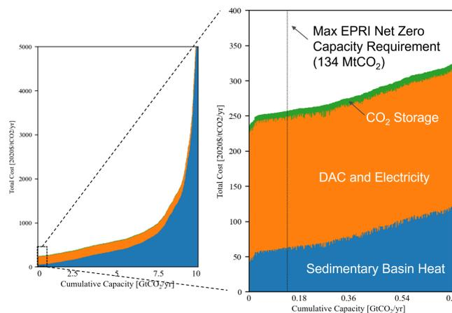
**Fig. 5: Supply Curves for Low-Temperature DAC.** The total capacity is limited by the geothermal heat availability and capacity of CO<sub>2</sub> storage because the sedimentary basin resource is “shared” between providing heat (i.e., brine) and storing CO<sub>2</sub>. The cost of DAC comprises most of the total cost until more expensive sedimentary basin heat resources are used.
