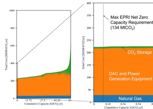
**Fig. 6: Supply Curves for High-Temperature DAC.** The total capacity is limited by the capacity of CO<sub>2</sub> storage because heat is provided by natural-gas. The cost of DAC comprises most of the total cost until the cost of CO<sub>2</sub> storage exponentially increases.
