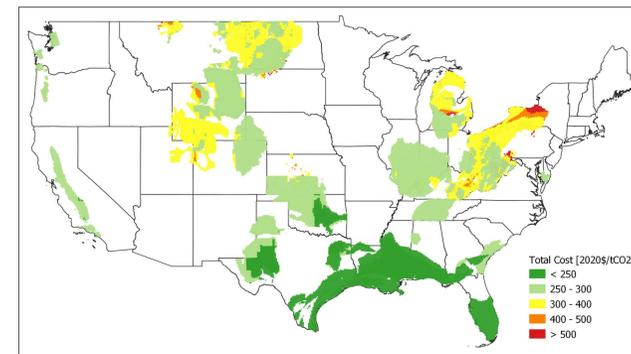
**Fig. 4: Geospatial Cost and Capacity of High-Temperature DAC.** Low-cost areas are those with the hottest air temperatures and highest relative humidity. Average annual air temperature and relative humidity data taken from [4].
